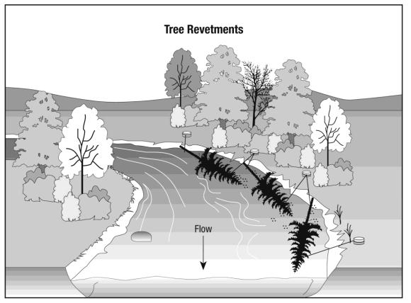
Figure 1. Conceptual drawing of tree revetments to protect stream bank from erosion (USDA, 1999).
